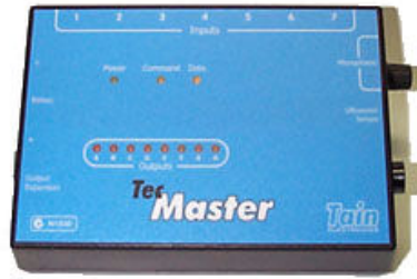
TecMaster Interface (7 inputs, 8 outputs) Cat. No. AD101 $580*
